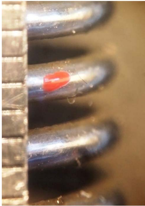
Figure 5. Image taken with camera through binocular loupe. The coils of the spring can be seen and to the left of the image the metal ruler used to measure the variations in length.
